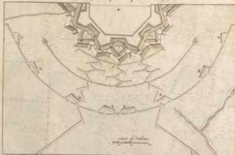
Fig. 3. Plan showing the disposition of the Batteries.
